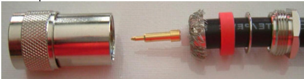
Slide barrel over cable, and tighten nut.
