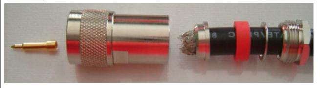
Fold braid back over the ferrule. Solder pin onto center conductor
